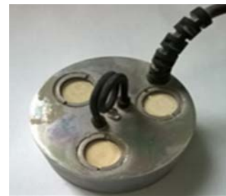
c. 1.7 MHz high-frequency ultrasonic atomizer
