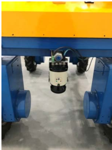
Figure 4 Installation location of the laser scanner
