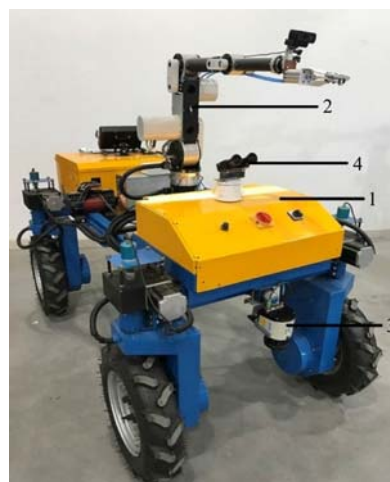
1. Moving chassis 2. Harvesting system 3. Navigation system 4. Vision system
