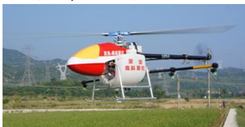
c. UAV HY-B-15L (battery powered UAV), Shenzhen Xinnong Gaoke
