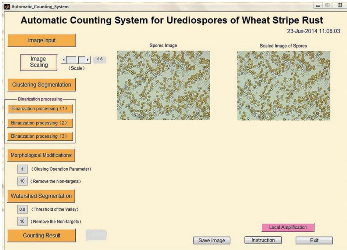
Figure 3 Realization of image input and image scaling for the automatic counting system
