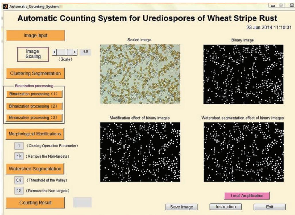
Figure 5 Morphological modification and watershed segmentation of spore microscopic image using the automatic counting system
