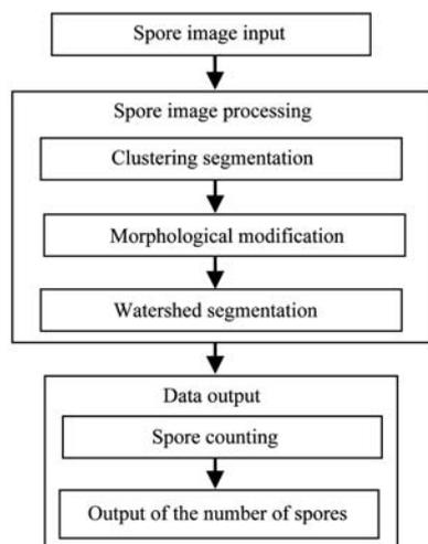
Figure 1 Main structural diagram of the automatic counting system for *Pst* urediospores
