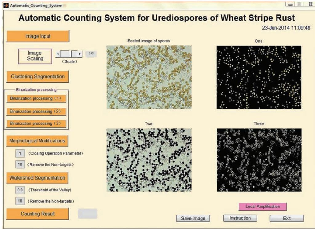
Figure 4 Realization of image segmentation for the automatic counting system
