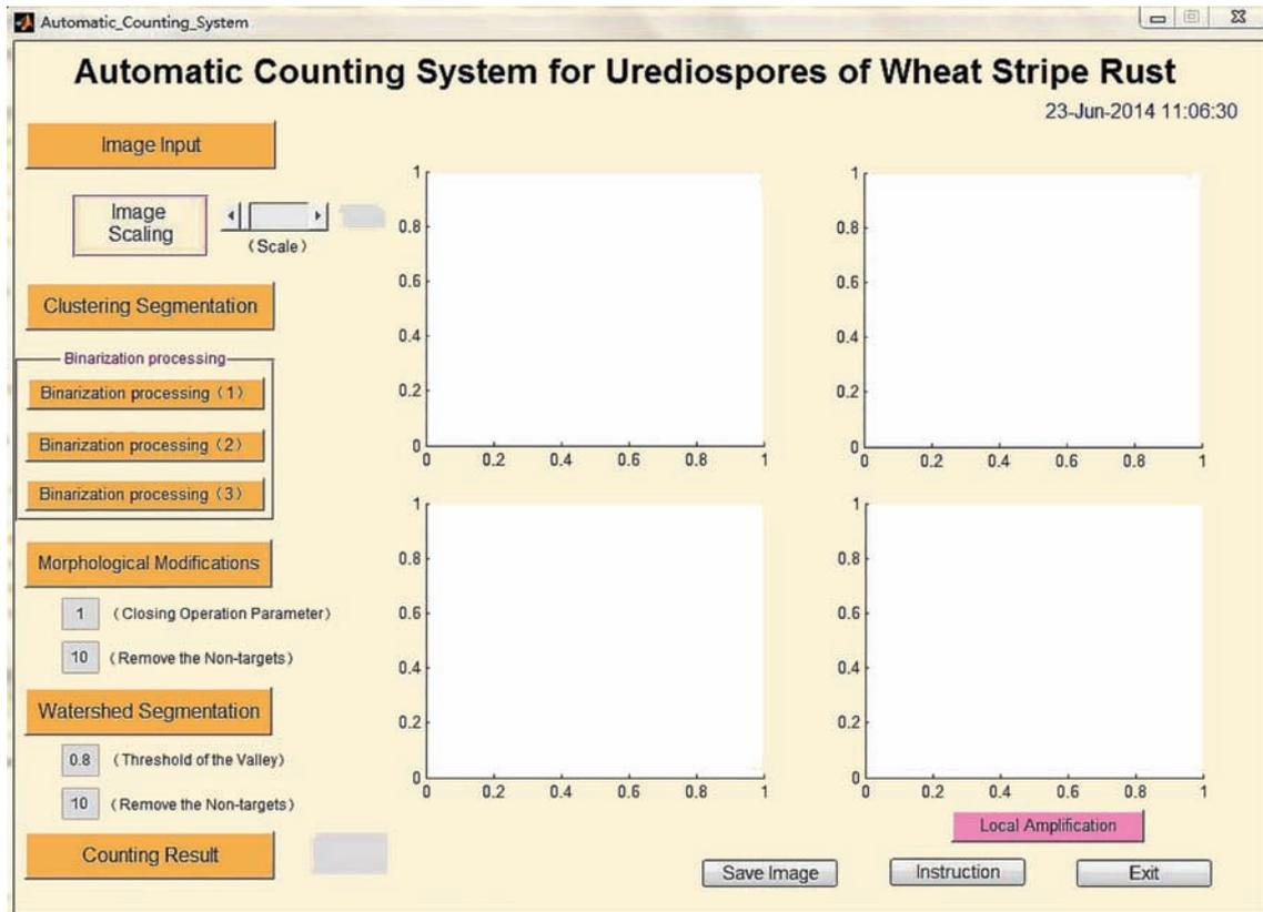
Figure 2 Graphical user interface of the automatic counting system for *Pst* urediospores
