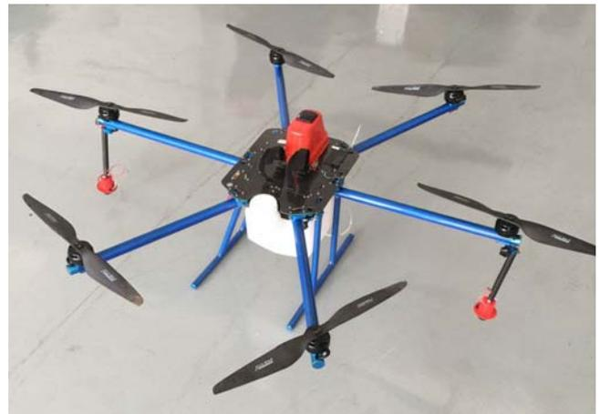
Figure 1 SLK-5 plant protection UAV
