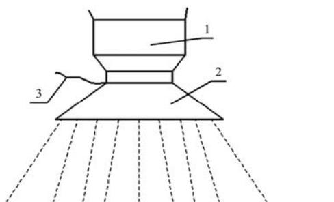
1. TR80-015C nozzle 2. Conical electrostatic electrode 3. Electrode wire
