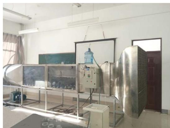
b. Site layout of droplet drift experiment
