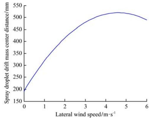
Figure 4 Effect of wind speed on droplet drift
