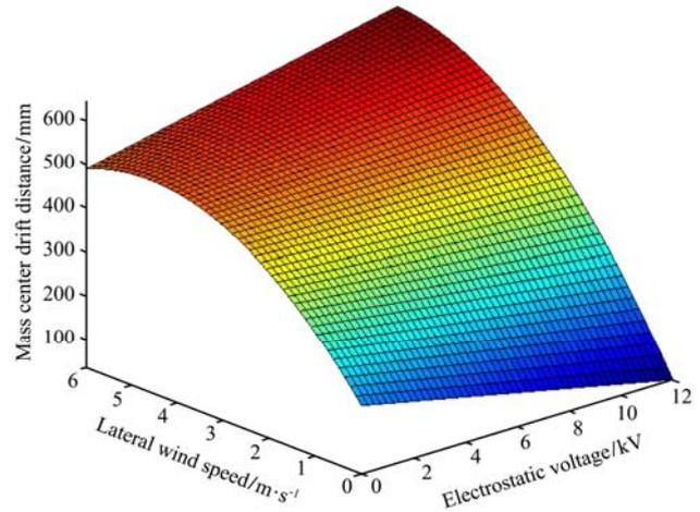
a. Response surface of droplet drift to electrostatic voltage and wind speed
