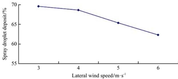
a. Droplet deposits in the test bed under different wind speeds
