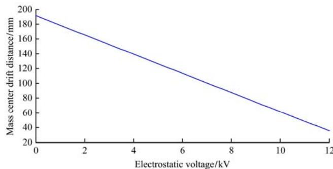
Figure 3 Effect of electrostatic voltage on droplet drift
