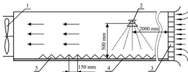
Note: 1. Fan 2. Electrostatic nozzle 3. Honeycomb air inlet 4. Artificial grass blanket 5. Droplet collector
