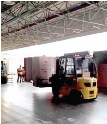
Figure 7 Measurement of slip distance of the target HCP from clamp arm through field test
