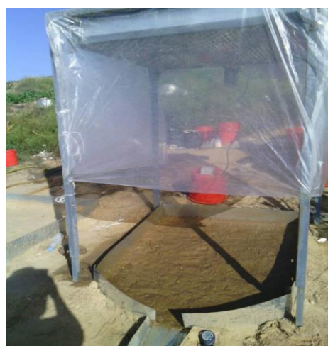
Figure 1 Simulation rainfall with a pinhole rainfall device in the experimental plot
