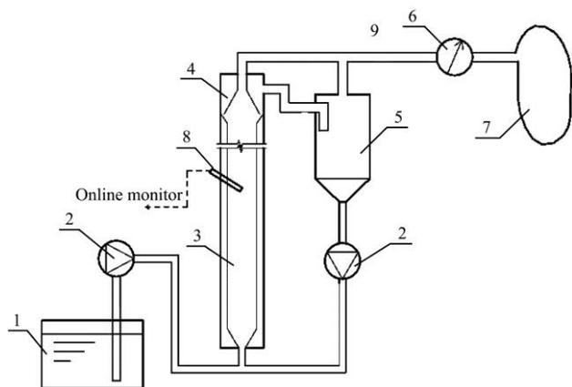
1. Pre-mixed tank 2. Peristaltic pump 3. Tubular photo-bioreactor
