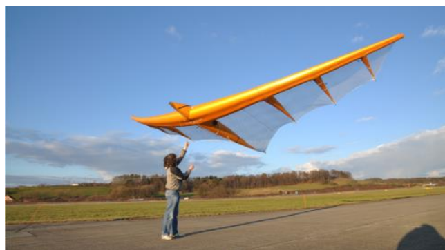
Figure 16 A tensairity kite in testing
