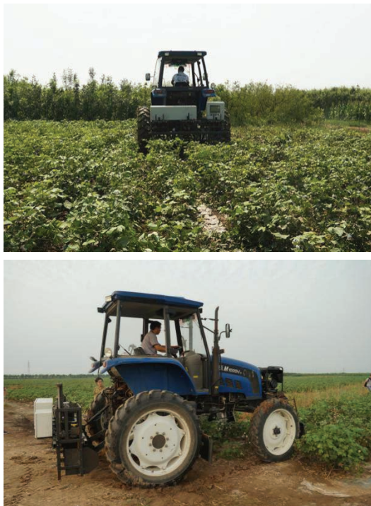
Figure 1 Self-developed cotton topper prototype attached to a tractor
