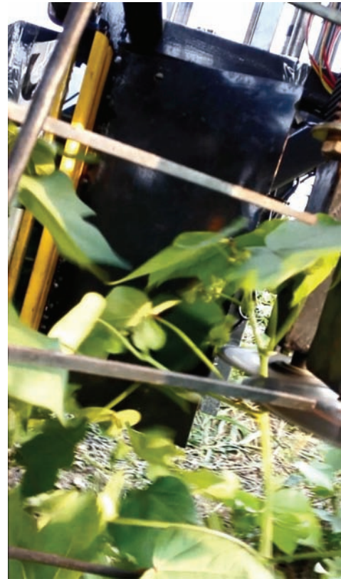
Figure 4 An example of the topper shearing a cotton top
