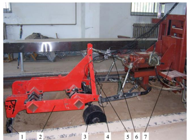
1. Subsoiler 2. Frame 3. Depth wheel 4. Right hanging pin sensor of CYB-601S 5. Left hanging pin sensor of CYB-601S 6. Upper link sensor of CYB-602S 7. Traction wagon
