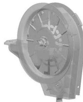
Figure 8 Geometric model of pickup finger precision maize seed metering device
