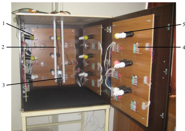
Note: 1. Tungsten 2. Camera carrier (Frame grabber) 3. Camera 4. LED 5. Fluorescent
