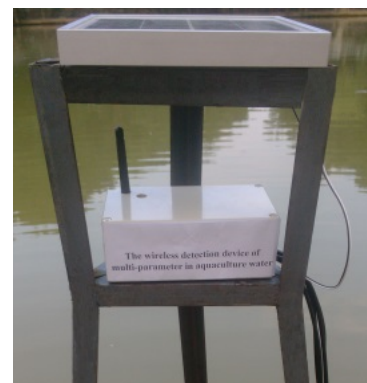
Figure 2 Actual sensor node of multi-parameters wireless detection system of water quality
