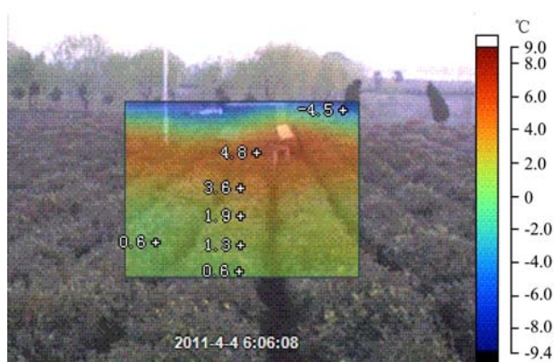
Figure 9 Thermal imagery of the area protected with JUVBF
