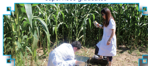
Inspecting the heavy metal contents of soil in field by rapid equipment
