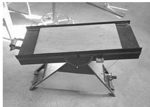
Figure 2 Device for determining the coefficient of static friction
