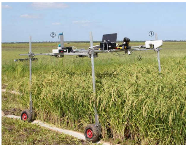
Figure 3 UGVs platform equipped with sensors working in paddy field
