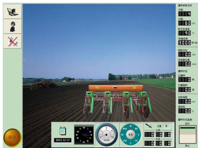
Figure 7 System interface for monitoring working status of planter
