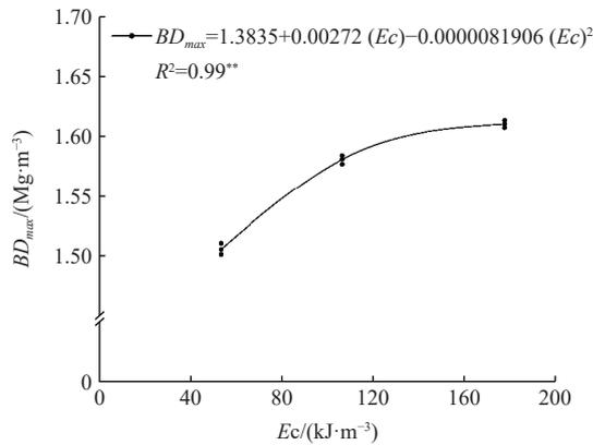
Figure 4 Fitting model equation of the change of the maximum dry bulk density  $BD_{max}$  with the compaction energy  $Ec$  of soil without straw cover after compacting in the Proctor test (\*\*The adjusted model was significant when  $p \leq 0.01$ )
