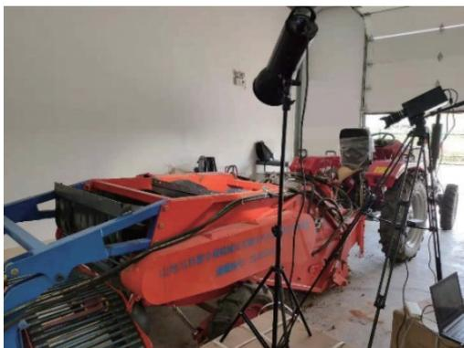
Figure 16 Bench test and high-speed photography layout plan
