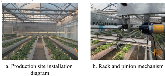
Figure 2 Installation of a movable LED supplementary lighting system in greenhouse strawberry production
