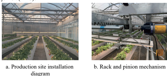
Figure 2 Installation of a movable LED supplementary lighting system in greenhouse strawberry production
