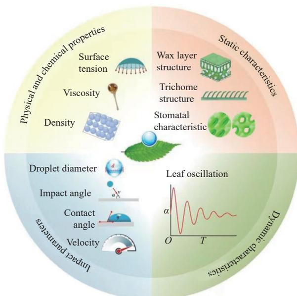
Figure 1 Factors affecting the droplet-foliage impact process
