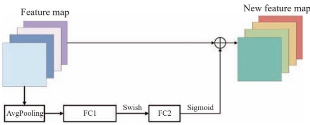
Figure 5 The structure of the SE
