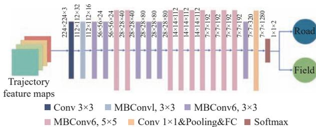
Figure 3 The network structure of EfficientNet-B0
