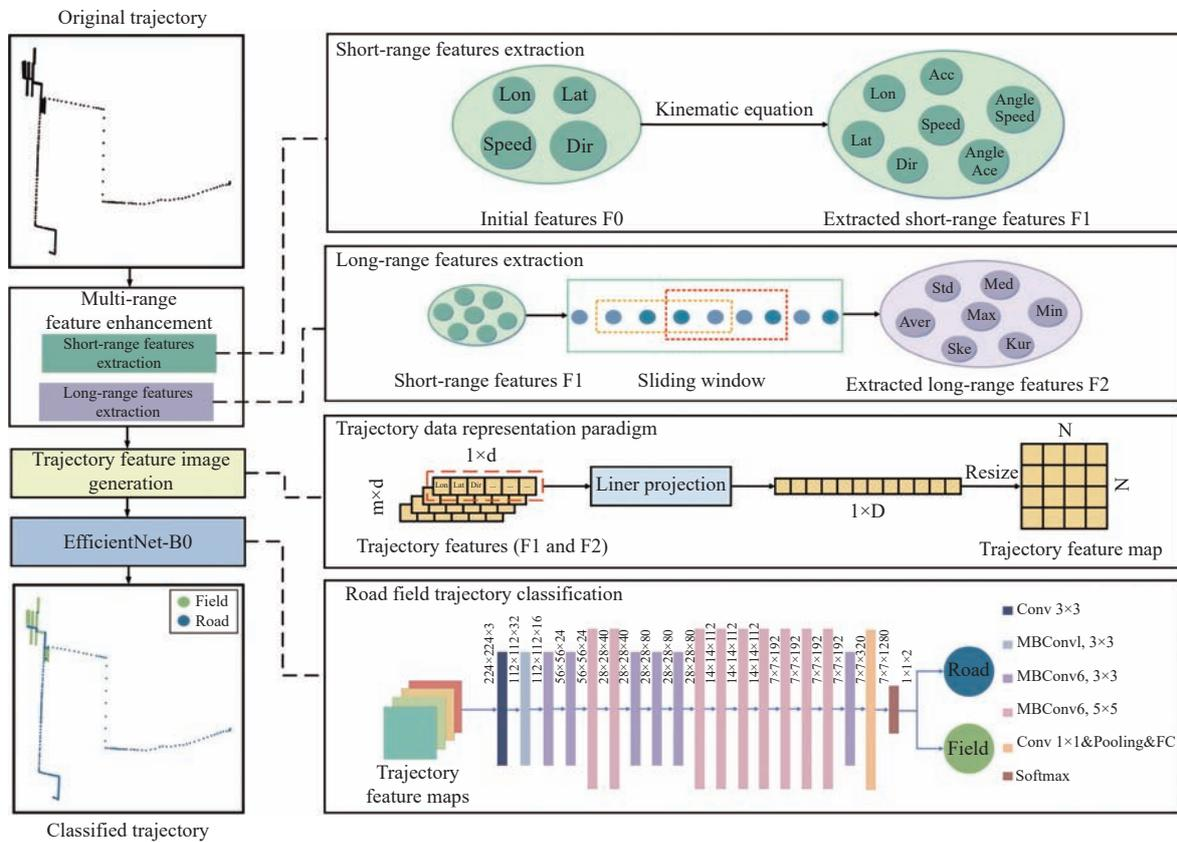
Figure 1 The pipeline of the proposed FDRNet
