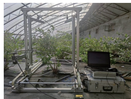
b. Vibratory picking test rig
