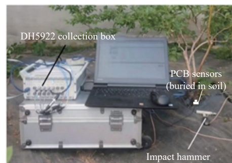
a. Test equipment
