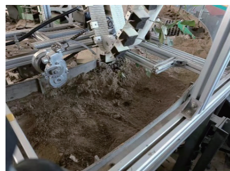
Figure 11 Test bench for sweet potato seedling
