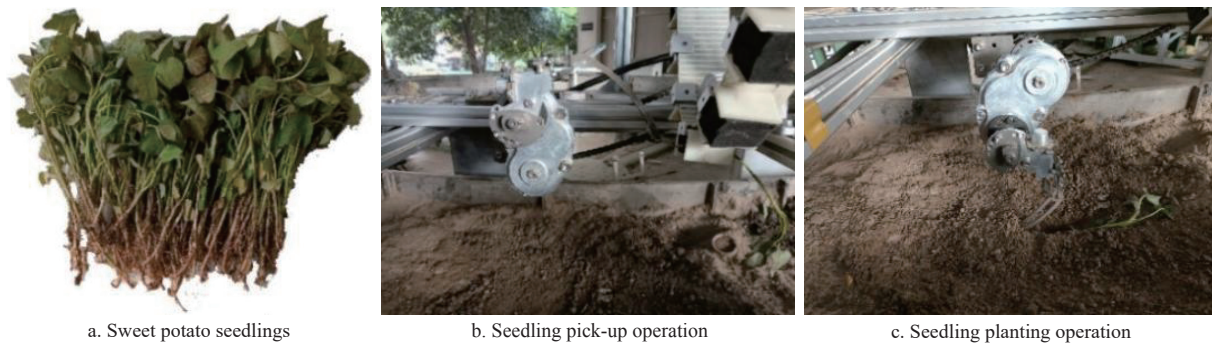
Figure 15 Transplanting tests for sweet potato seedling
