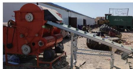
Figure 13 Operation validation of the wind sieve type cleaning device
