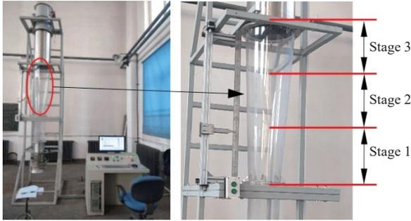
Figure 2 WXS-1 agricultural material suspension experiment bench
