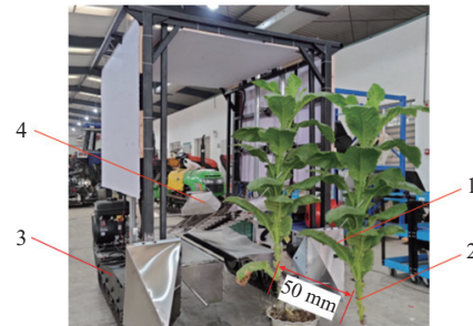
1. Tobacco; 2. Smoke sticks; 3. Tracked chassis; 4. Comb picking device
