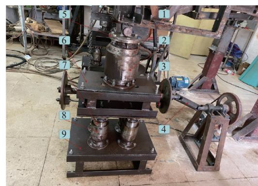
1, 2. External and the internal sleeves of the upper spring 3. Eccentric mass blocks 4. Axis coupler 5, 6, 9. Upper, middle and lower support platforms 7, 8. External and the internal sleeves of a lower spring
