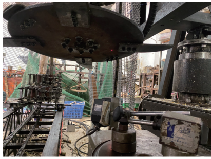
a. The laser of the LK-G150 laser displacement sensor falling on the cutter along the z axis to measure the axial cutter vibration amplitude
