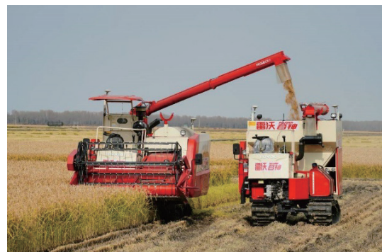
Figure 2 Cooperative operation of unmanned combine harvester and grain truck
