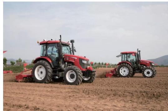
Figure 1 Master-slave tracking operation of tractor unit
