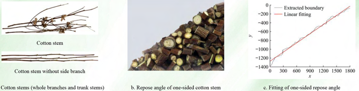
Figure 1 Repose angle of one-sided cotton stem and fitting of repose angle \alpha
