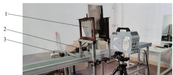
1. fertilizer applicator with spiral fluted roller 2. fertilizer box 3. conveyor belt
