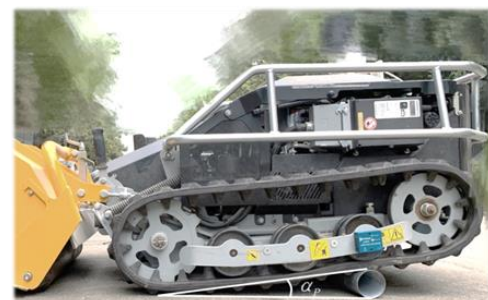
Figure 13 Road surface excitation test process
