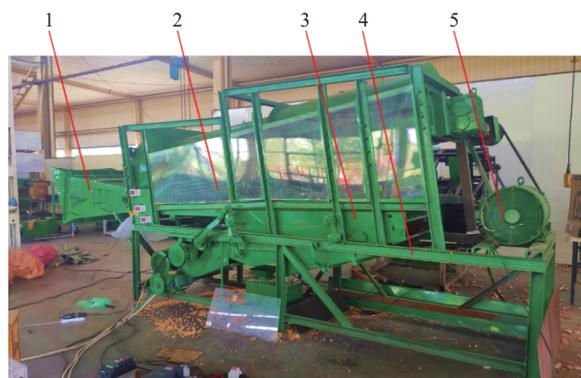
1. Maize feeding device 2. Threshing device 3. Cleaning device 4. Frame 5. Power-driven system
