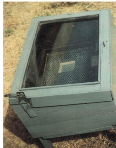
Figure 1 Picture of a direct passive solar dryer
