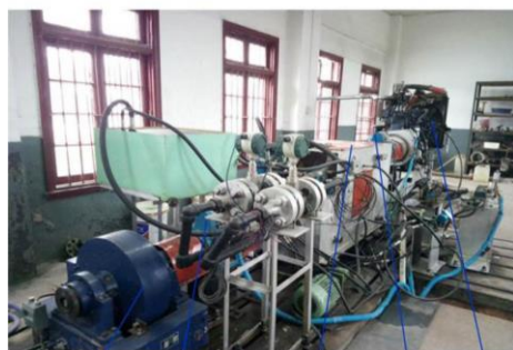
1. Dynamometer 2,4. Speed torque sensor 3. HMCVT 5. Engine
