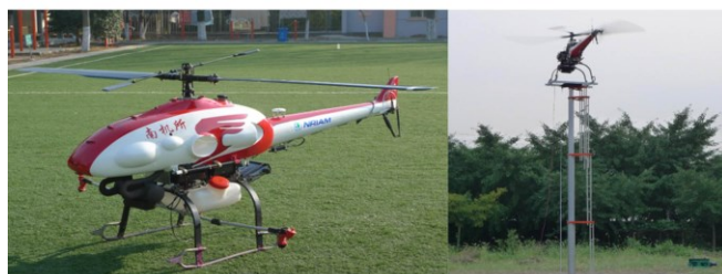
Figure 3 Tested CPUAS Z-3N and experimental installation
