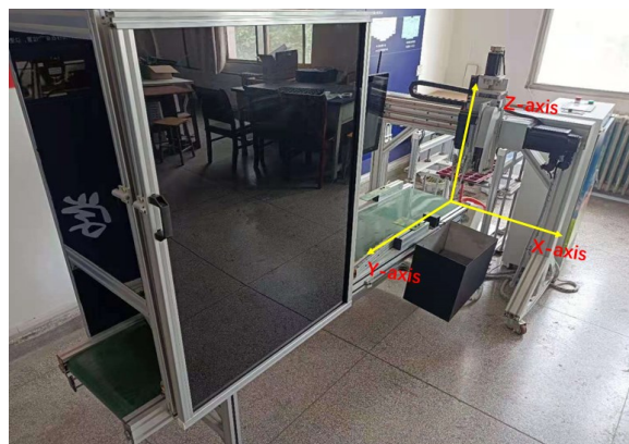
Figure 3 Intelligent sorting and transplanting device for healthy vegetable seedlings
