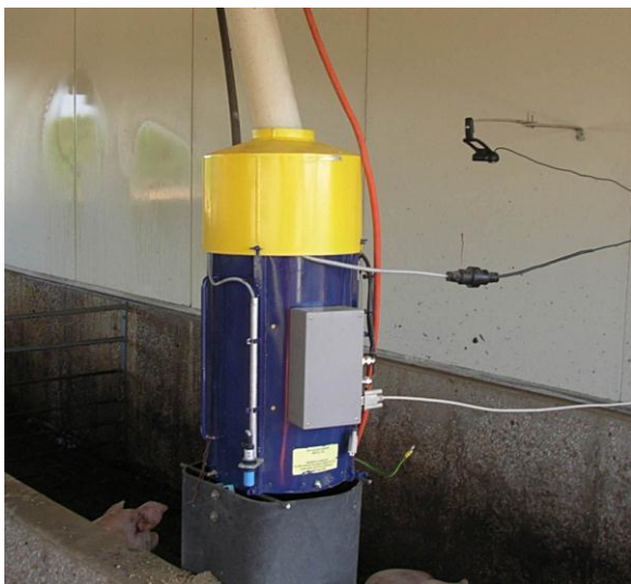
Figure 4 Prototype feed sensor and the camera system undergoing testing at a commercial piggery site [22]
