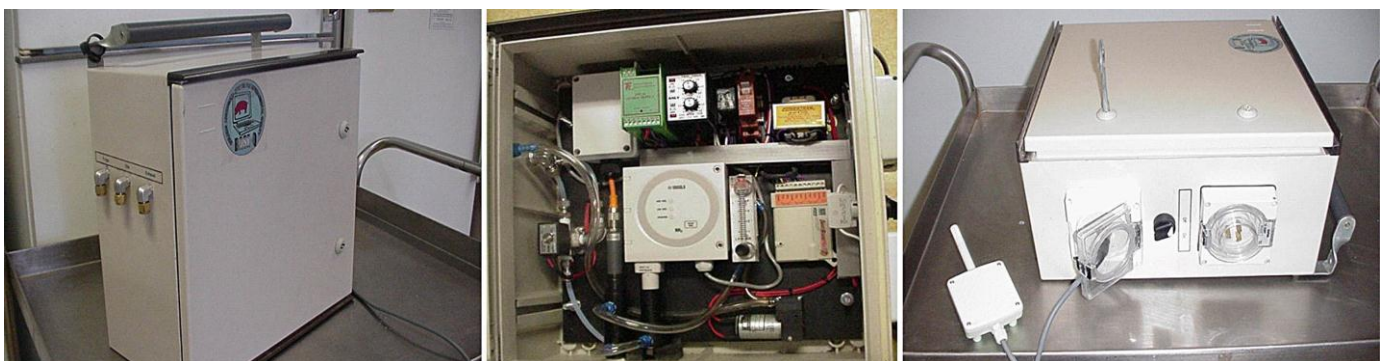
Figure 5 Environmental monitoring modules of the BASE-Q system [24]
