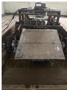
Figure 8 Soil bin test device
