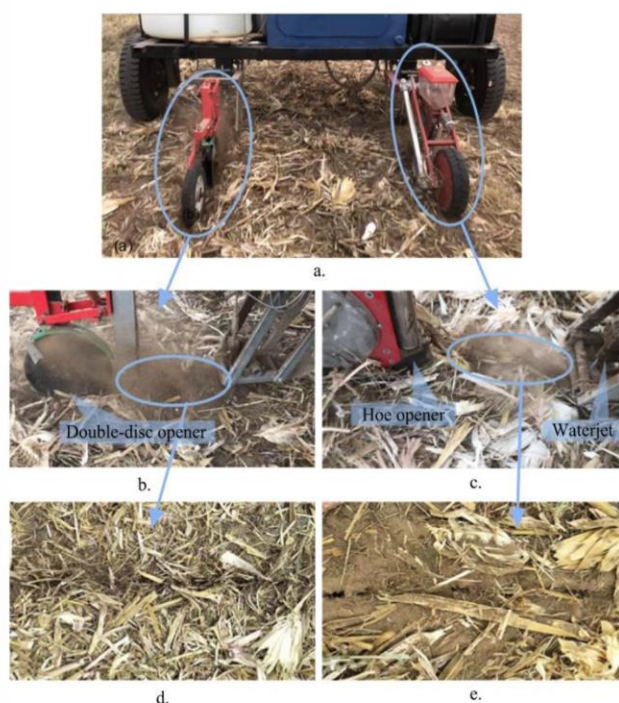
Figure 3 Field experiments for different type of furrow opener coordinate with UHP waterjet
