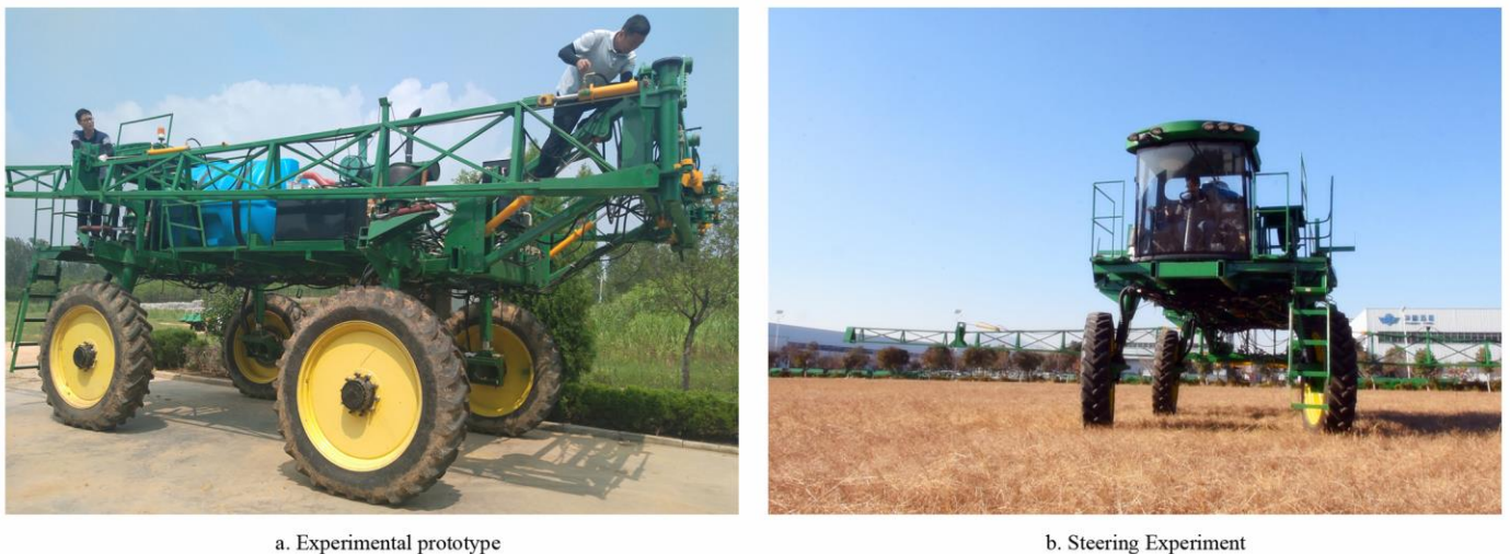
Figure 12 Performance experiment of sprayer chassis
