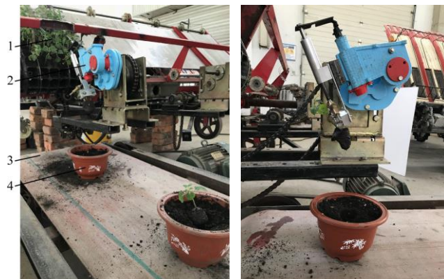
a. 45° view of the test prototype b. Front view of the test prototype 1. Salvia splendens seedlings 2. Transplanting mechanism 3. Conveyor belt 4. Flowerpot
