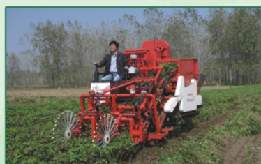
Fig. 5. Half-feed quad-row peanut combine harvester
