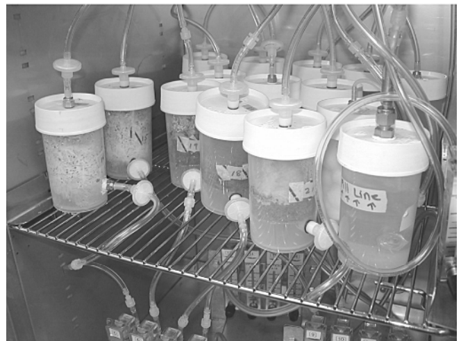
Figure 1 Incubator (30~32°C, air flow at 20 ml/min) with tomato pomace in reactors.
