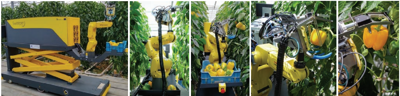
Figure 1 SWEEPER robot in action: The world first fully automated sweet pepper harvesting platform
