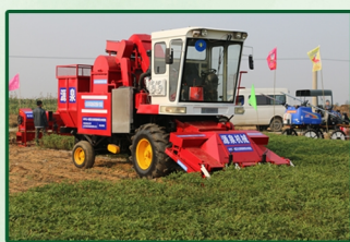
4HYGJ-6, the world's first peanut harvester both peanut and stalks were harvested.
