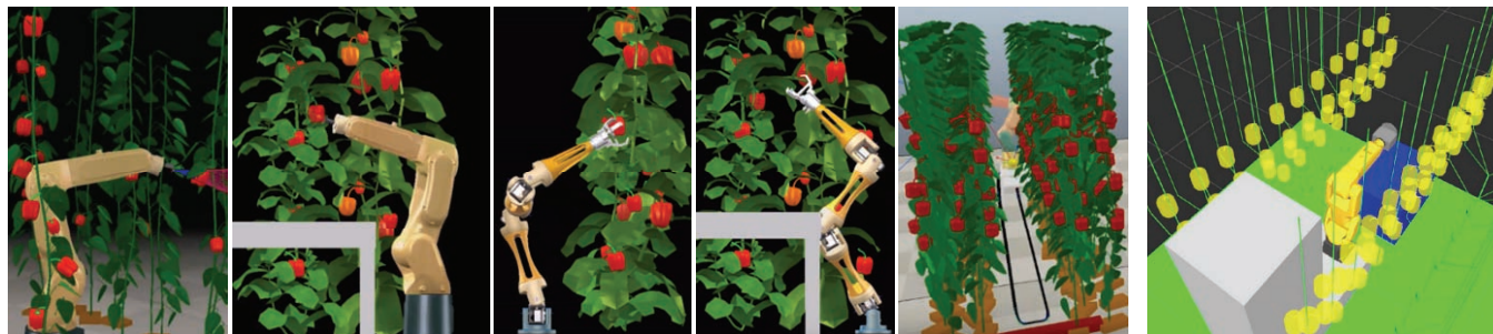
a. V-REP scene [1] visualized in Rviz using vision sensor publisher (robot control and image processing in MATLAB) Source: AdaptiveAgroTech.com b. ROS MoveIt and RViz Source: sweeper-robot.eu
