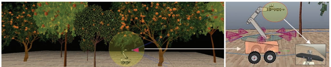
a. Simulation environment for the virtual citrus orchard and the prototype field robot with multiple sensors and obstacle avoidance
