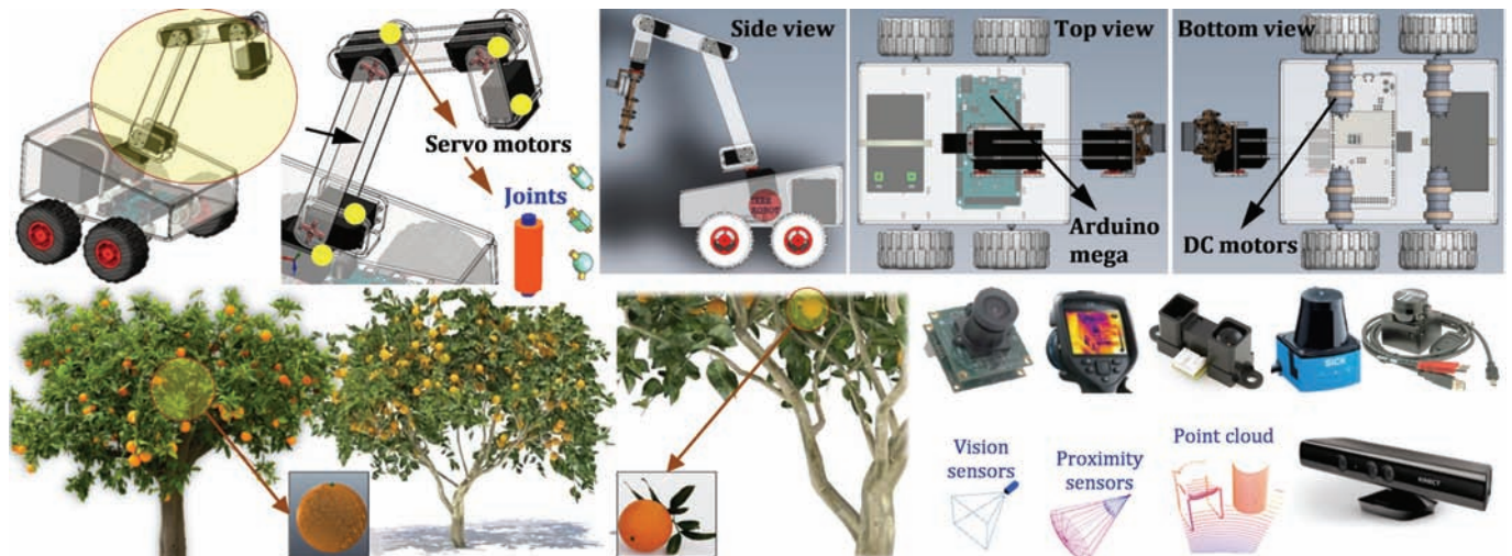
Figure 12 Major scene objects used in the V-REP case study simulation, including CAD model of a prototype robot platform, artificial citrus trees, and simulated sensors
