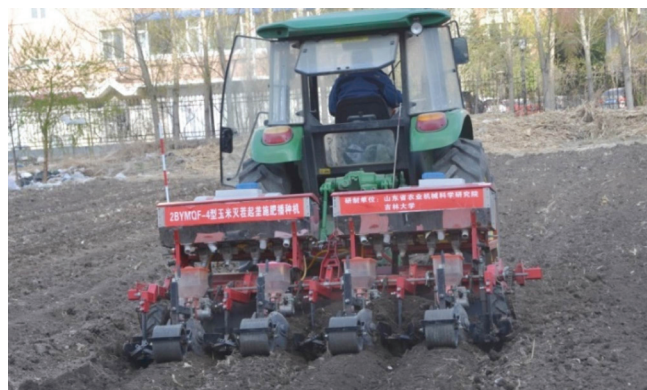
Figure 4 2BYMQF-4 maize seeder with the seed furrow liquid spraying device. Four levels of water volume and two types of nozzle were set in the experiments
