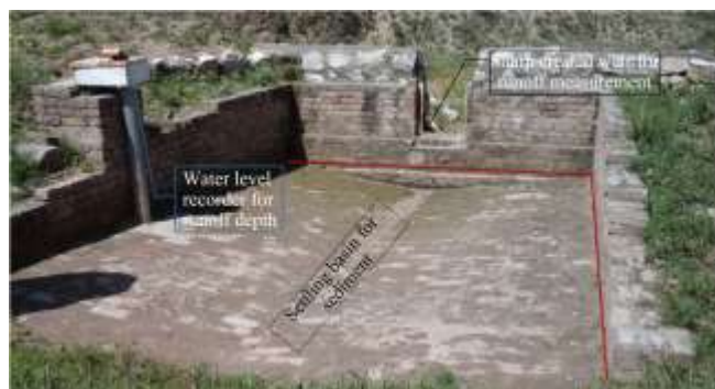
Figure 5 Experimental setup for runoff and sediment yield
